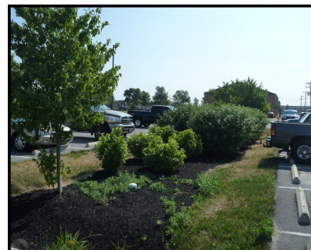
Left: Bioretention ponds are an excellent opportunity to reflect native ecosystems. Use native vegetation and take advantage of natural features. Right: Medians between parking aisles can be planted with trees and native wetland vegetation to collect and filter runoff.
